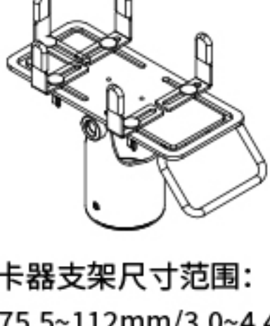
刷卡器支架尺寸范围: W(75.5~112mm/3.0~4.4inch) D(180~219mm/7.1~8.6inch) H(35~80mm/1.4~3.1inch)
